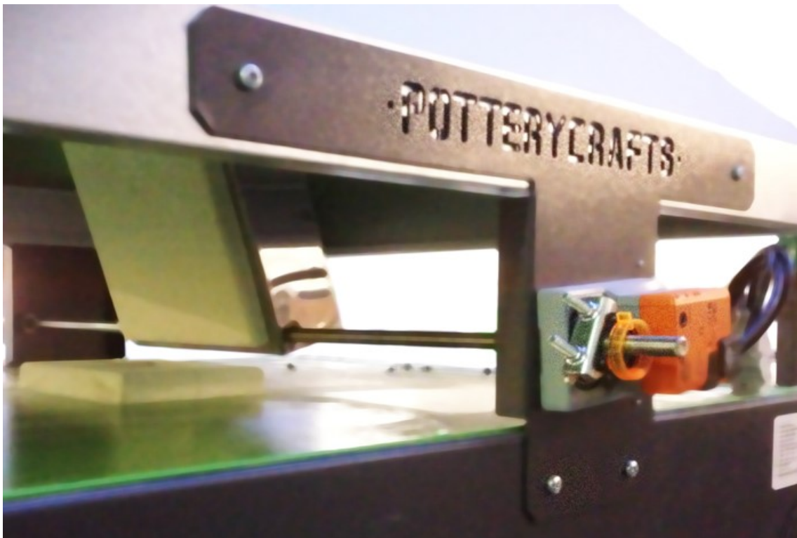
Pictured is the P5943 kiln with added ventilation hood and automated damper.
